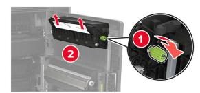
**3** Open the standard trays, and then remove the jammed paper.
