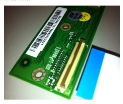
**3** Place your finger in the middle of the actuator, and then rotate the locking actuator to the locked position.
