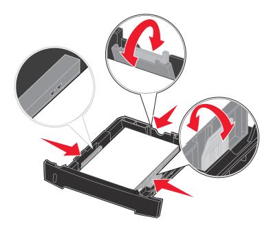
**Note:** Load letterhead paper with the design side facing down. The top edge of the sheet with the logo should be placed at the front of the tray.
