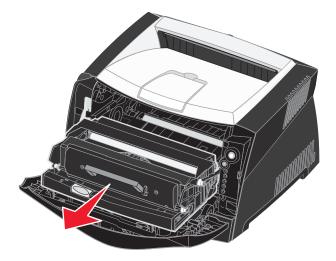
Place the print cartridge assembly on a flat, clean surface.
