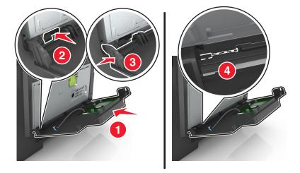
**10** Run the ISP cable through the controller board shield door.
