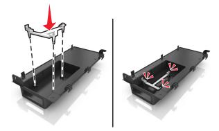
**5** Slide and push the ISP solution into the plastic bracket.
