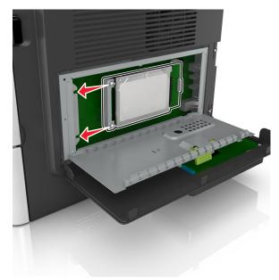
**c** Tighten the two screws.
