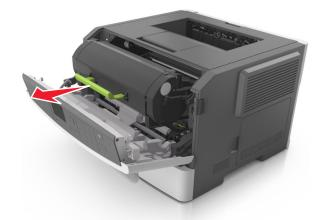
**3** Lift the green handle, and then pull the imaging unit out of the printer.
