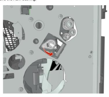
**12** Pry the pointed end of the 2nd pickup pushing to release the locking pin underneath.
