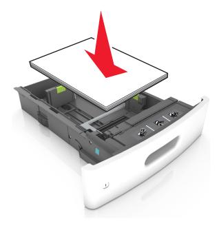
• Make sure the paper is below the solid line, which is the maximum paper fill indicator.
