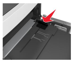
**Note:** Use the paper size indicators on the bottom of the tray to help position the guides.
