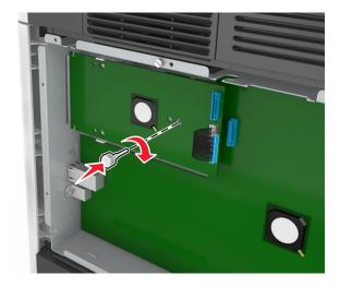
**Note:** Turn the screw clockwise, enough to hold the ISP in place, but do not tighten it yet.
