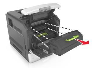
**3** Lift the green handle, and then pull out the imaging unit from the printer.
