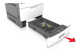
**2** Squeeze and slide the width guide to the correct position for the size of the paper being loaded until it *clicks* into place.
