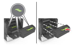
**Warning—Potential Damage:** When replacing a toner cartridge, do not leave the imaging unit exposed to direct light for an extended period of time. Extended exposure to light may cause print quality problems.
