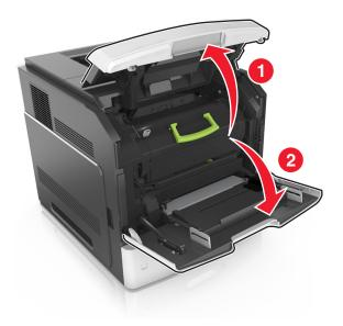
**2** Pull the cartridge out of the printer using the handle.
