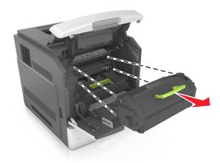
**3** Unpack the new toner cartridge, then remove the packing material, and then shake the cartridge to redistribute the toner.
