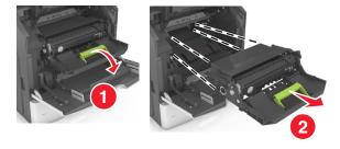
Warning—Potential Damage: Do not expose the imaging unit to direct light for more than 10 minutes. Extended exposure to light may cause print quality problems.
