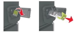
**3** Open the staple guard, and then remove the loose staples.
