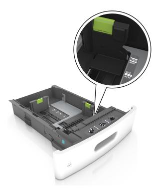
**3** Unlock the length guide, and then squeeze and slide the guide to the correct position for the size of the paper being loaded.
