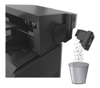
**3** Insert the emptied hole punch box back into the finisher until it *clicks* into place.
