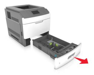
**2** Squeeze and slide the width guide to the correct position for the size of the paper being loaded until it *clicks* into place.
