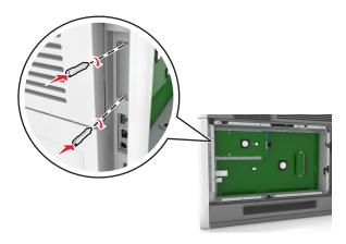
**10** Tighten the thumbscrew that is attached to the ISP.
