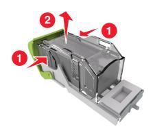
**4** Insert the front side of the new staple case into the staple cartridge, and then push the rear side into the cartridge.
