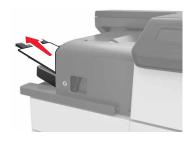
Press the latch on the staple finisher, and then slide the finisher to the left.
