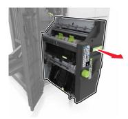
**5** Remove the jammed paper from any of the following locations: **Note:** Make sure that all paper fragments are removed.
