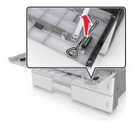
The controller board supports one optional Lexmark Internal Solutions Port (ISP). Install an ISP for additional connectivity options.
