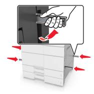
**7** Align the printer with the tray, and then lower the printer into place.
