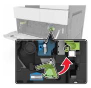
**4** Remove the photoconductor unit.
