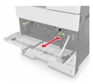
**5** Remove the printhead wiper.
