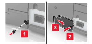
**2** Remove the screws from the controller board access cover.
