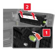
**3** Open the standard trays, and then locate the jammed paper.
