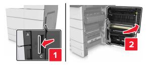
Note: If the 3000-sheet tray is installed, then slide the tray to the right to open the door.
