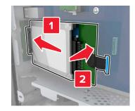
**b** Use the two provided screws to attach the hard disk mounting bracket.
