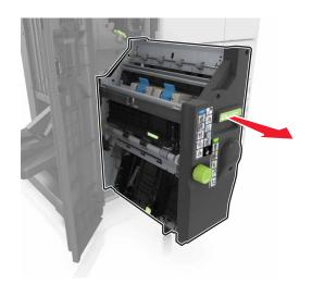
5 Remove the jammed paper from any of the following locations:Note: Make sure that all paper fragments are removed.
