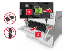
**3** Unlock the photoconductor unit.
