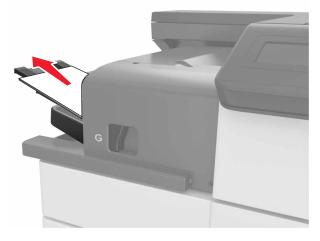
**2** Press the latch and slide the staple finisher to the left, and then remove the jammed paper.
