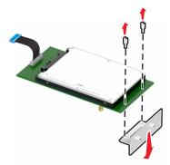
**b** Align the standoffs of the hard disk to the holes in the ISP, and then press the hard disk down until the standoffs are in place.
