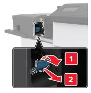
**3** Remove the empty staple cartridge from the cartridge holder.
