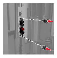
7 Insert the plug of the ISP interface cable into the connector of the controller board.
