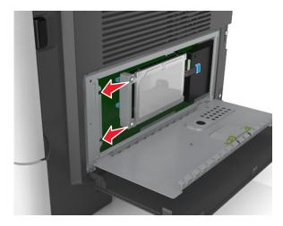
**d** Tighten the two screws.
