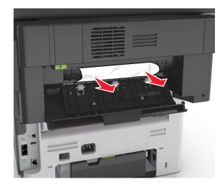
Open the finisher trap door, remove any paper fragments inside the trap door.
