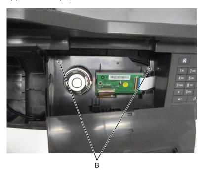
**6** Remove the two screws (C) securing the control panel assembly to the scanner assembly.
