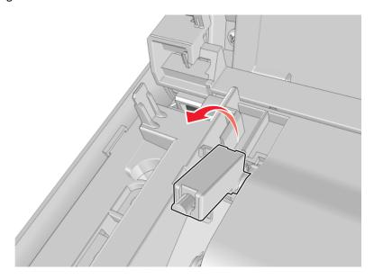
**3** Twist and then remove the cartridge plunger.
