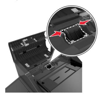
Pull away the separator roll and remove.
