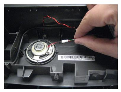
**8** Feed the speaker cable through the channel on the right side of the printer.
