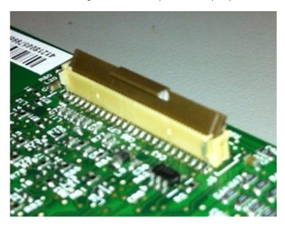
2 Insert the cable with the contacts on the cable away from the locking actuator. Insert the cable on top of the actuator.
