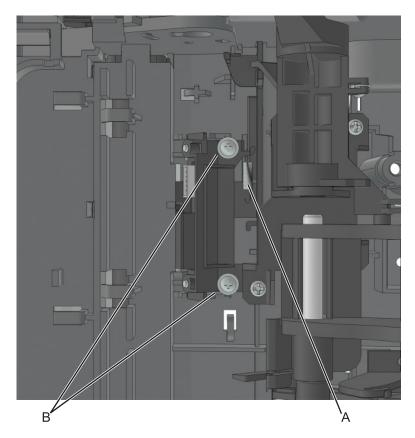
**9** Disconnect the cable from the sensor.
