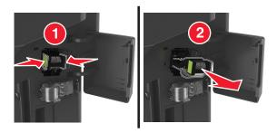
Lift the staple guard, and then remove any jammed or loose staples.
