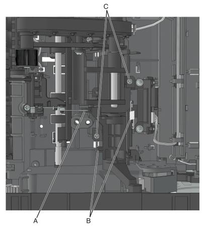
Below are the cam release and bracket.
