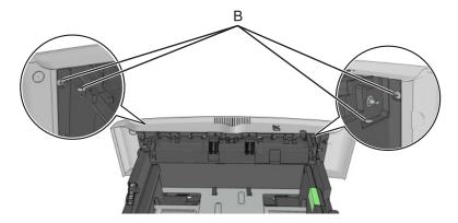
Push out the top part of the drawer cover, and then remove the separator roll assembly.
