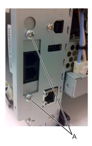
**5** Lift the modem to release, and then remove.
