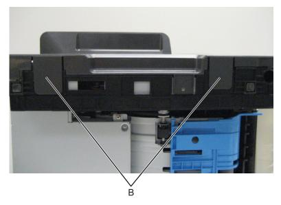
Pull the cover forward, and remove it from the printer.
