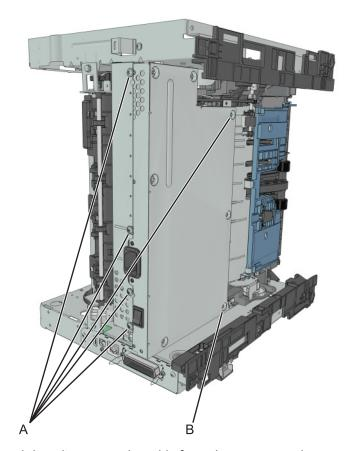
**6** Remove the power supply, and then disconnect the cable from the power supply.
