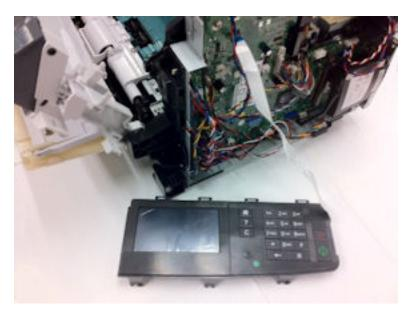
After installing the LSU, perform the mechanical and electronic LSU adjustments with the printer in this configuration. When the LSU is properly adjusted, re-install the control panel assembly to the scanner, and then re-install the scanner assembly to the MFP.
