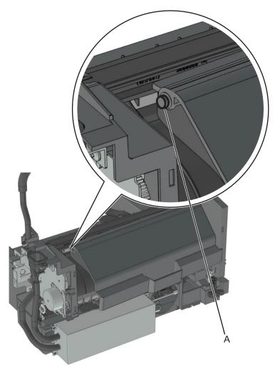
**2** Using a flat-blade screwdriver, release the latches, then remove the input cover.
