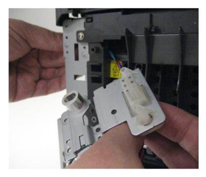
7 Using a pair of pliers, squeeze the nylon mounts to dislodge the stapler connector, and remove the stapler cable.
