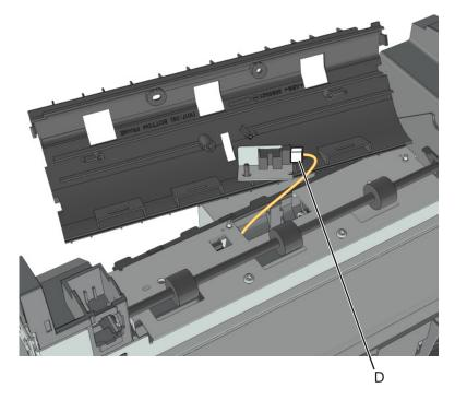
**6** Release the latches, and then remove the sensor.
