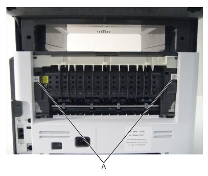
**3** Lift the upper portion of the machine to release the cover, and then remove the cover.
