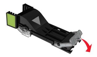
Insert stapler cartridge back into the finisher until it *clicks* into place.
