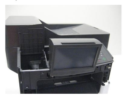
Remove the two screws (B) behind the display.
