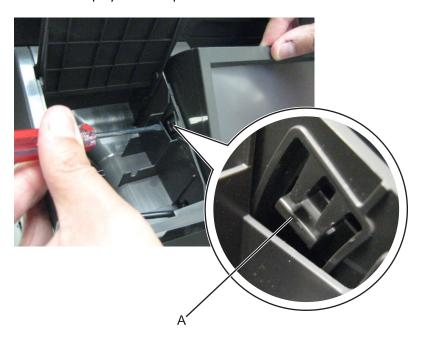
Position the display at the angle shown to access the screws behind it.
