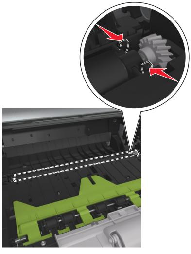
**2** Lift to remove the transfer roll.
