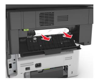
Open the finisher trap door, and then remove any paper fragments from inside the trap door.
