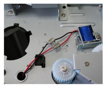
**d** Route the cable using the new path, and secure it with a cable tie (C).
