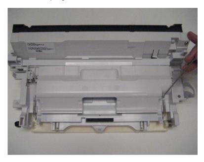
**3** Disconnect the left and right MPF links from the front access cover.
