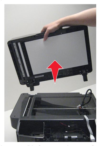
**Installation note:** After the new ADF is installed, perform scanner manual registration, see **"Scanner manual registration"** on page 205 and scanner calibration, see **"Scanner calibration"** on page 181.
