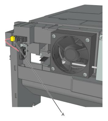
Release the latches, and pull the sensor off the stapler.
