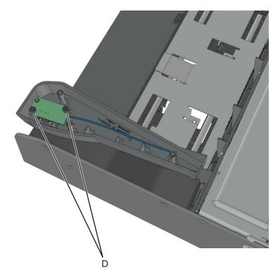
**11** Route the sensor cable off the stapler, then remove the sensor.
