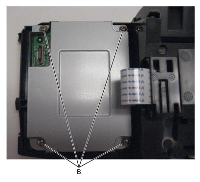
Disconnect the UICC video cable from the UICC card.
