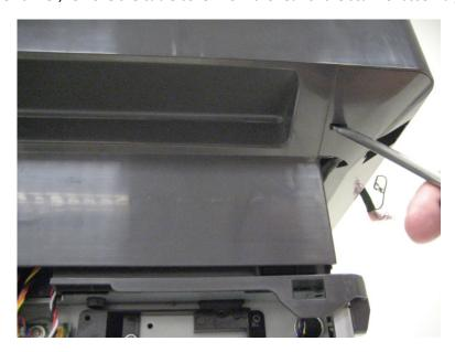
**3** Remove the scanner assembly from the MFP.
