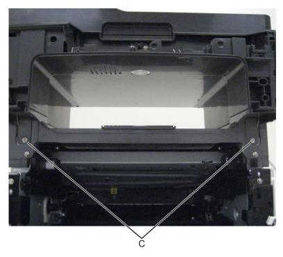
**12** Lift the complete scanner assembly away from the printer, and remove.
