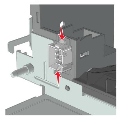
**6** Route the cable off the stapler, and remove.
