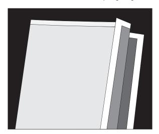
**4** If the grid lines of the right flap align below the corresponding lines on the left flap, then adjust the printhead clockwise relative to the printer, and recheck. If the grid lines of the left flap align below the corresponding lines of the right side, then adjust the printhead counterclockwise.
