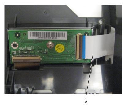
Place the control panel assembly facedown on a non-marring surface.
