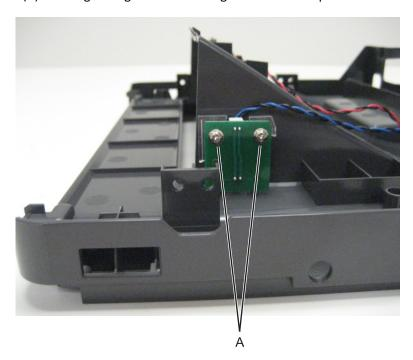
**3** Disconnect the cable (J1) from the sensor.
