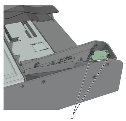
Route the sensor cable off the stapler, then remove the sensor.
