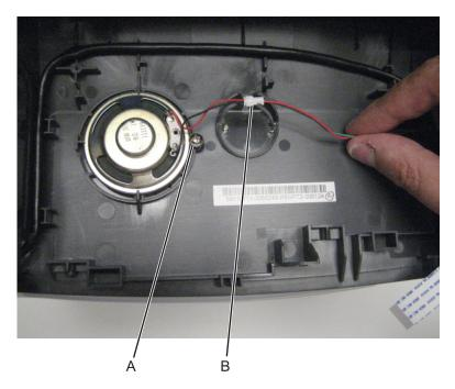
**4** Gently slide the speaker to the right, and remove it from the scanner assembly.
