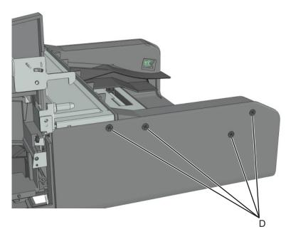
Lift the cover, then release the cables routed through the top cover.
