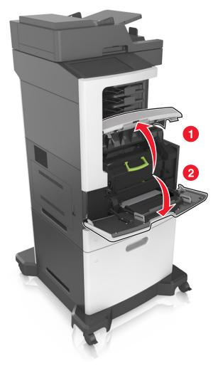
**2** Lift the green handle, and then pull out the toner cartridge from the printer.
