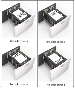
• If you are loading prepunched paper for use with the staple finisher, then make sure the holes on the long edge of the paper are on the right side of the tray.
