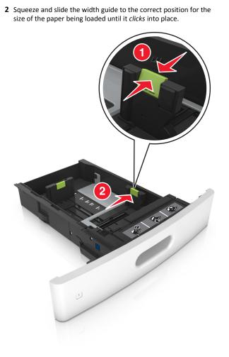
**Note:** Use the paper size indicators on the bottom of the tray to help position the guides.
