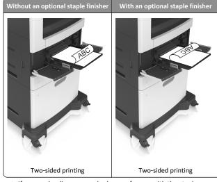
• If you are loading prepunched paper for use with the staple finisher, then make sure the holes on the long edge of the paper are on the right side of the tray.
