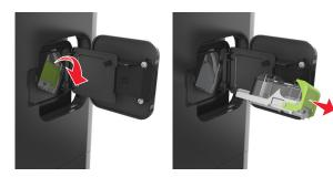
**4** Use the metal tab to lift the staple guard, and then remove any loose staples.
