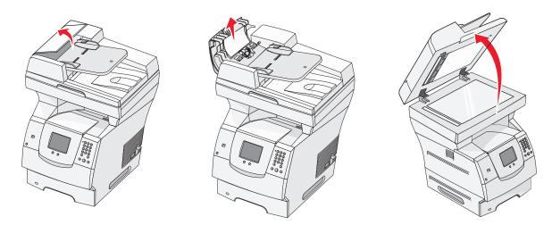
4 Open the scan unit access door, and remove any jammed pages.
