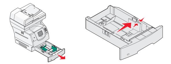
**3** Squeeze the rear guide tab, and slide the guide to the correct position for the size media you are loading.
