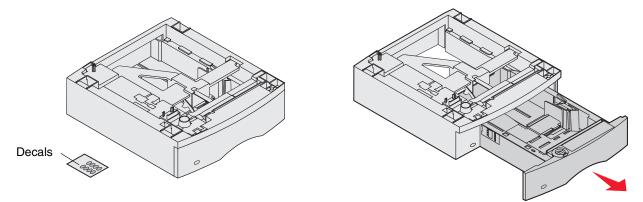
2 Place the support unit on top of any previously installed drawers or the table or MFP cabinet where you plan to use the MFP.
