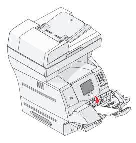
8 Set the Paper Size and Paper Type for the envelope feeder to the correct value for the print media you loaded. See Setting the Paper Type and Paper Size for more information.
