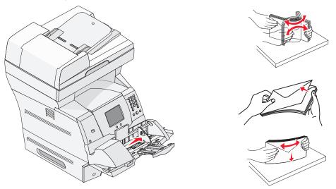
**5** Load the stack of envelopes flap side down with the stamp area and the flap on the left. The end of the envelopes with the stamp area enters the envelope feeder first.
