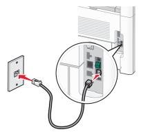
**3** Remove the protective plug from the EXT port  $\widehat{\text{III}}$  of the printer.
