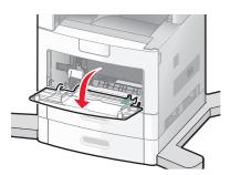
**2** Using the handle, pull the multipurpose feeder extender.
