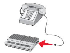
**5** Connect a third telephone cord from the answering machine to the EXT port in of the printer.
