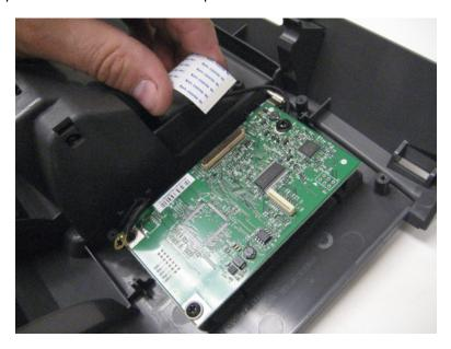
**8** Remove the four screws (B) securing the control panel board (7" tilting display) to the control panel.
