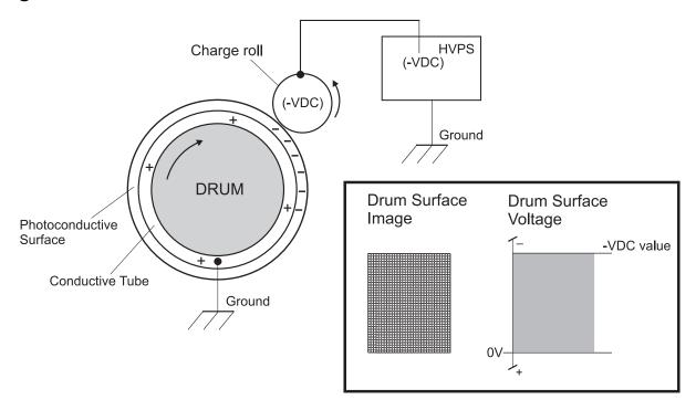
The charge roller places a uniform negative electrostatic charge on the surface of the drum. The drum surface is made of a photoconductive material that holds an electrical charge as long as the drum remains in darkness. Light striking the drum discharges the surface charge.
