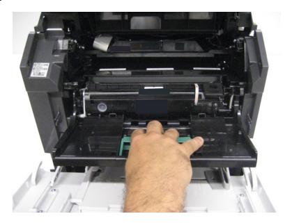
Using the drive gear, gently pull the right side of the transfer roller to slightly detach it from the machine.
