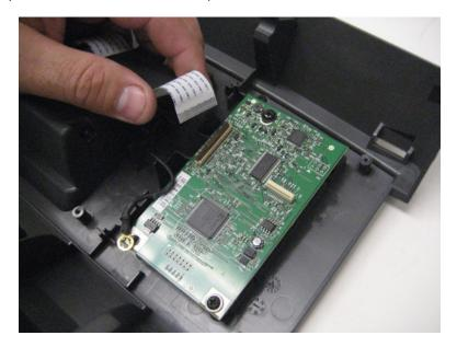
**8** Remove the four screws (B) securing the 4.3" tilting display to the control panel.
