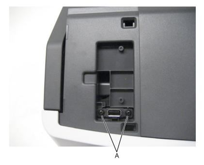
Release the USB cable from the control panel and pull it out and slightly away.
