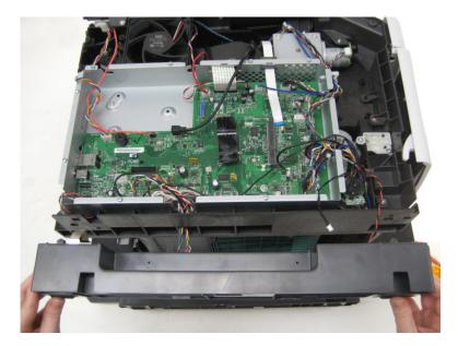
**10** Disconnect the three cables from the controller board.
