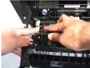
**3** Pull the fuser access door away from the machine to remove it.
