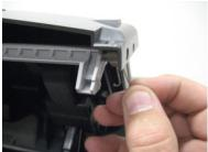
**4** Carefully flex the corner of the control panel frame as shown in the following image.
