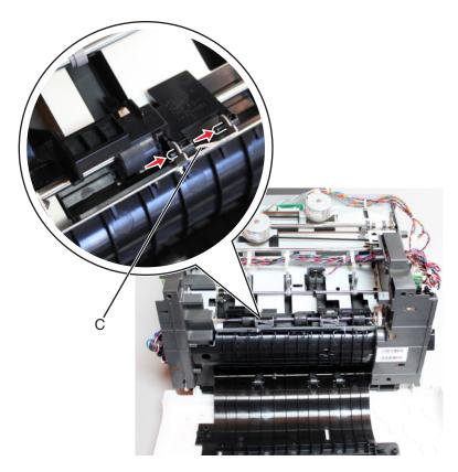
**6** Ease the media stack flap off the stapler assembly.
