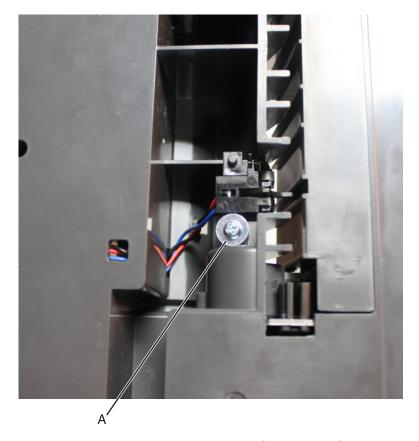
**6** Release the cable from its cable holders, then remove the sensor (pass through).
