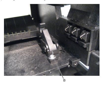
**15** Remove the transfer roller right arm.
