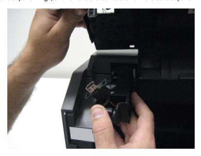
**7** Remove the screw (C) securing the grounding cable to the machine.
