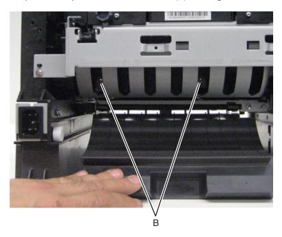
**5** Gently but firmly pull the LVPS partially from the machine, as shown in the following image.
