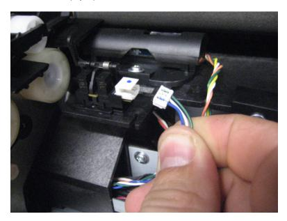
**13** Release the hooks (A) securing the sensor (input) to the machine.
