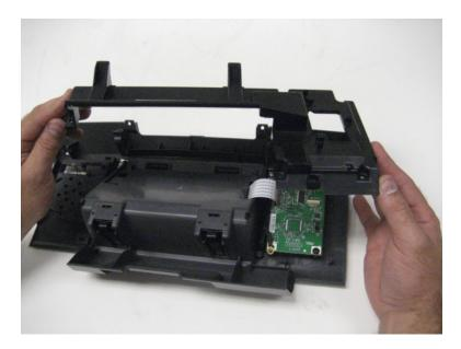
Disconnect the display ribbon cable from the control panel board.
