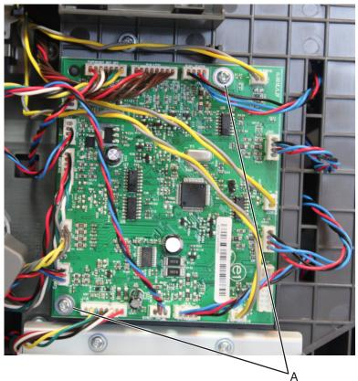
4 Remove the controller PCBA.
