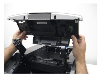
Installation warning: When replacing the control panel, ensure that all cables are properly reconnected.
