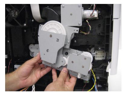
Disconnect the cable from the main drive motor.
