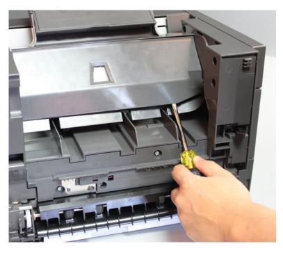
2 Release the latches (A) to remove the LED clear lens. Disconnect the cable (B), and remove the standard output bin LED.
