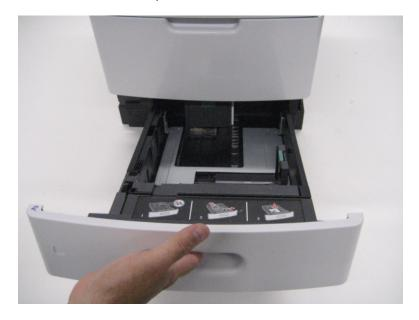
**2** Lift the media tray, as shown in the following image, and remove it from the machine.
