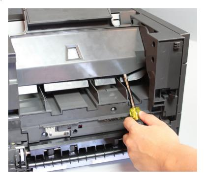
**3** Release the latches holding the sensor (B) to the cover.
