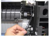
Return the printer to the normal position, and remove the duplex motor.
