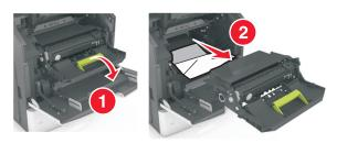
**5** Place the imaging unit aside on a flat, smooth surface.
