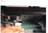
**Note:** When removing the pick roller assembly, avoid all contact with the roller surfaces, or paper jams might occur.
