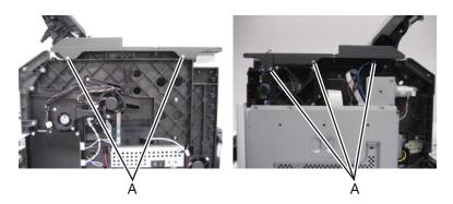
**9** Carefully detach the control panel ribbon cable from the standard bin cover.
