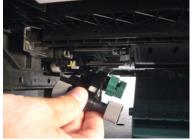
Note: When replacing the pick rollers, do not touch the roller surfaces, or paper jams might occur.
