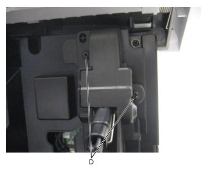
**12** Remove the right control panel hinge.
