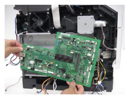
**Installation note:** Make sure you retain the flash card from the original controller board so that you can use it with the replacement controller board.
