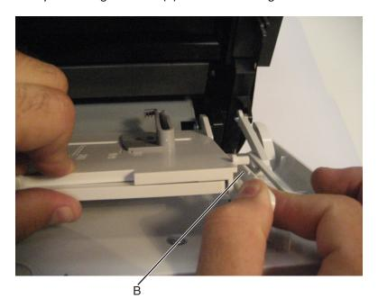
Raise the MPF tray to a vertical position, and detach it from the machine.
