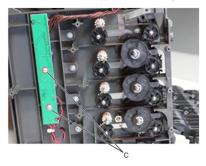
Disconnect the two cables (D), and remove the output bin LED assembly.
