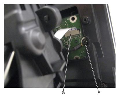
Remove the control panel.
