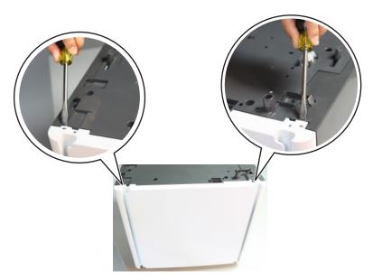
**3** Ease the drawer assembly rear cover off the drawer, and remove.
