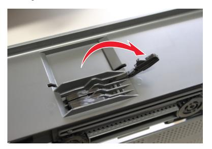
**3** Press the free end to remove the actuator.
