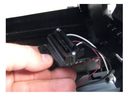
Remove the screw (B) securing the transfer roller right arm to the machine.
