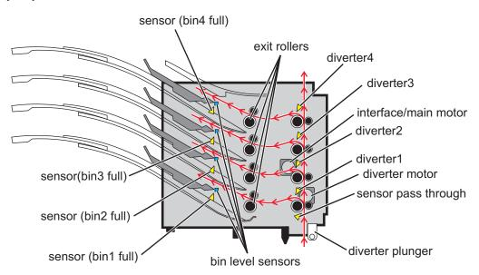
When the mailbox is installed on top of the printer, the diverter plunger changes the position of the diverter below it. Since the diverter position of the printer below is opened, the printed paper will be re-routed. Instead of exiting the standard output bin, the media enters the mailbox. The movement of the diverter plunger can be controlled by its diverter motor, depending on the printer's commands.
