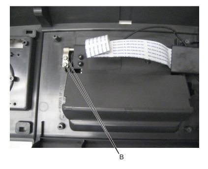
**9** Remove the 4.3" tilting display from the control panel.
