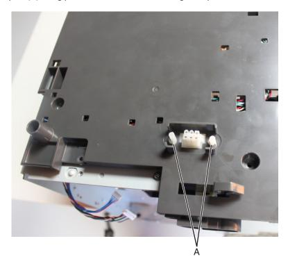
**5** Route the interface cable off the drawer, and remove.
