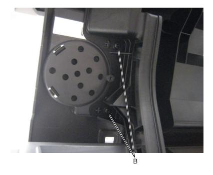
**6** Disconnect the left control panel hinge, and remove the USB cable from the control panel.
