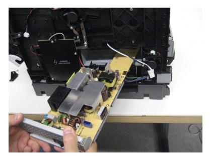
**Installation warning:** When replacing the LVPS, ensure that the LVPS is perfectly square to the printer, as opposed to replacing it at an angle. If you try to replace the LVPS at an angle, damage will occur to the controller board.
