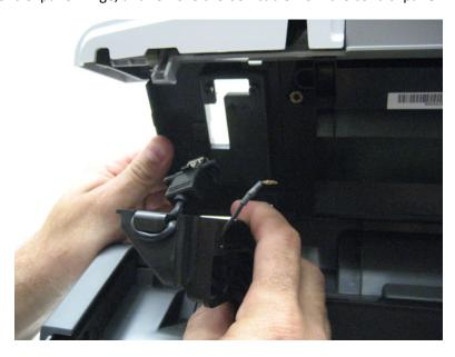
**9** Remove the screw (D) securing the plastic cap to the machine.
