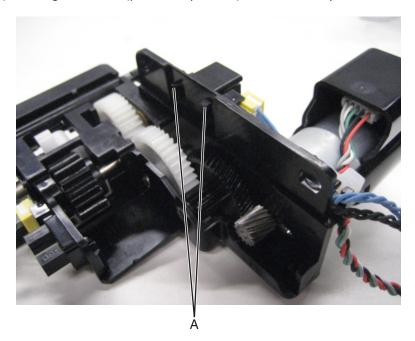
**9** Remove the sensor (pick roller position).
