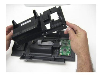
7 Disconnect the display ribbon cable from the control panel board.
