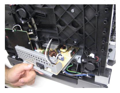
Disconnect the fuser power cable (C) from the LVPS.
