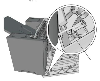
**Note:** Fasten the string to the rear side to prevent it from recoiling into the interior of the HCOE.
