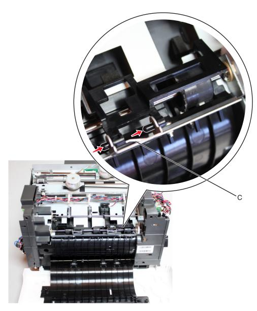
Ease the media stack flap off the stapler assembly.
