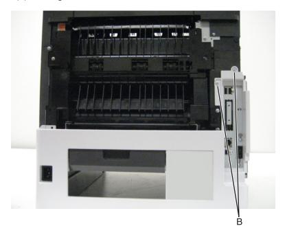
Gently pull the rear lower cover up and out to remove it.
