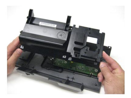
Remove the three screws (B) securing the control panel board (7" tilting display) to the control panel.
