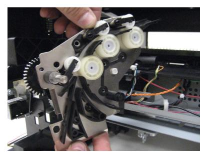
Warning—Potential Damage: When removing the media aligner, ensure that you retain the attached spring.
