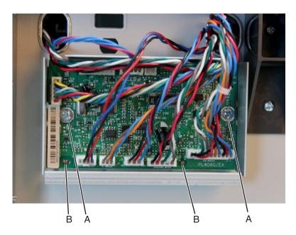
4 Remove the controller PCBA.
