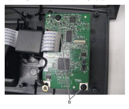
9 Remove the control panel board.
