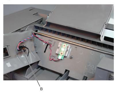
**4** Disconnect the cable from the stapler controller PCBA, then remove the sensor (finisher bin media present).
