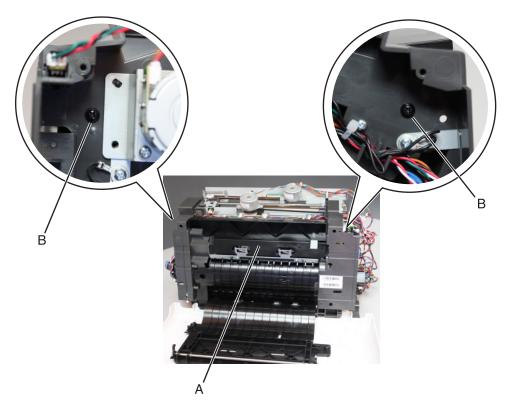
**5** Move the media stack flap to the right to release the pins from the holes.
