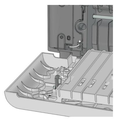
Remove the two screws (B), then remove the right cover.
