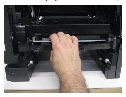
**Warning—Potential Damage:** When you press down the plate, you are lowering the pick pad (B) away from the MPF feed roller to prevent damage. If you do not do this, the pick pad will likely become damaged.
