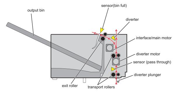
When the output expander is installed on top of the printer, the diverter plunger changes the position of the diverter below it. Since the diverter position of the printer below is opened, the printed paper will be re-routed. Instead of exiting the standard output bin, the media enters the output expander. The movement of the diverter plunger can be controlled by its diverter motor, depending on the printer's commands.
