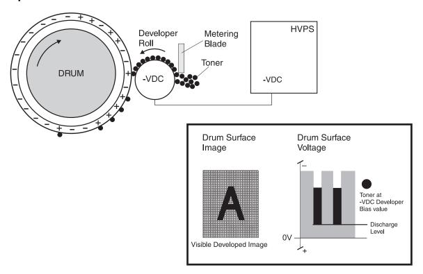
The toner contained within the PC cartridge has an electrical property that causes it to adhere to the development roller. The metering blade spreads the toner into a very thin layer on the development roller. Friction between the development roller and the CM blade development roller generates a small electrical charge that is transferred to the toner.
