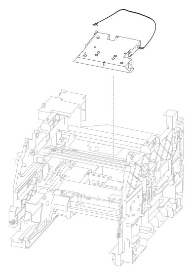
The printhead scans the photoconductor drum surface with a laser beam. It consists of four components: laser diode (LD) card assembly, printhead motor, polygon mirror, and the start of scan card assembly.
