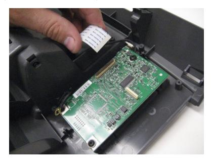
**8** Remove the four screws (B) securing the 7" tilting display to the control panel.
