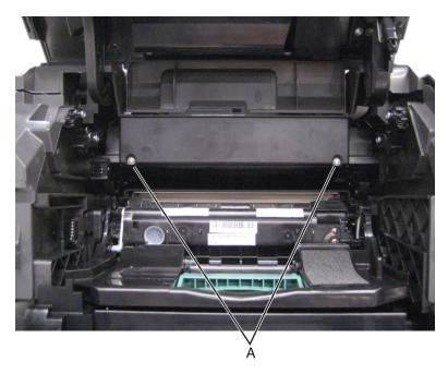
**Warning—Potential Damage:** When removing the printhead access cover, ensure that the cartridge cooling fan cable does not become disconnected.
