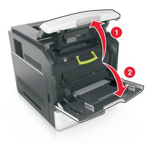
**2** Lift the green handle, and then pull the toner cartridge out of the printer.
