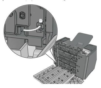
**2** Position the door to an angle approximately 90 degrees from the expander, then remove.
