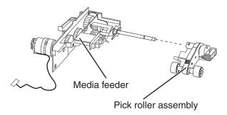
The pick roller assembly which is part of the media feeder, is a mechanical unit supplying media from the media tray to the paper path. The driving force from the media feeder drive motor, is transmitted to the two pick rollers to feed media from the tray and is also used to lift the tray plate that is used to lift the media stack into contact with the pick rollers.
