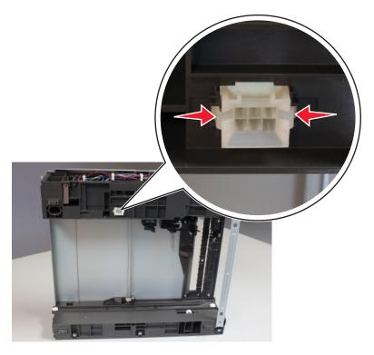
**6** Route the interface cable off the drawer, and remove.
