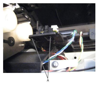
14 Remove the sensor (input).
