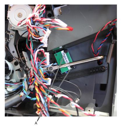
Disconnect the cable (B), and remove the sensor (bin full receive).
