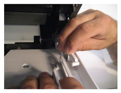
**5** Slide the front door to the left, and detach it from the machine.
