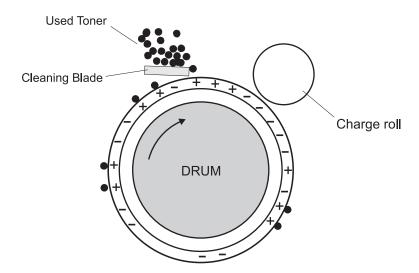
The cleaning blade removes any toner that remains on the drum after the transfer process. The toner that the cleaning blade removes is collected inside the sealed PC cartridge.
