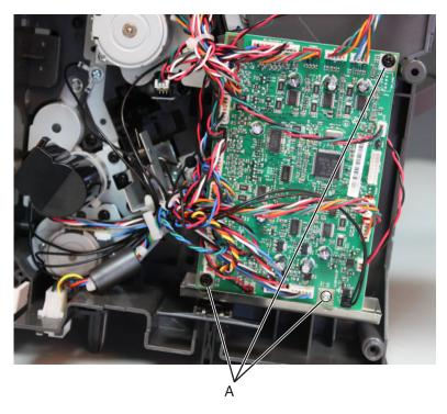
**3** Remove the controller PCBA.
