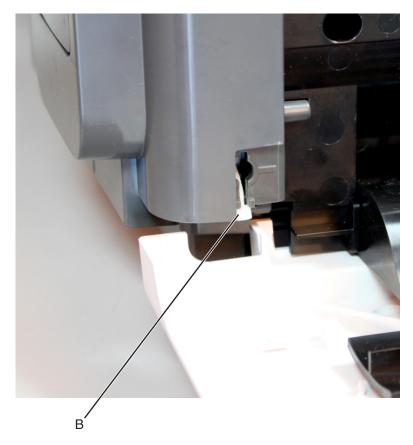
2 Position the door at an angle approximately 90 degrees from the stapler. Release the right hinge of the door first (1), then move the door to the right (2) to release the left hinge.
