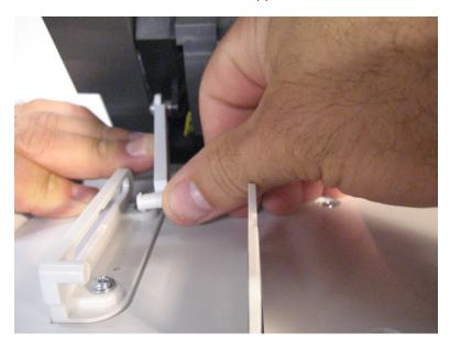
4 Gently flex the right bracket and release the tab on the MPF support link, as shown in the following image.
