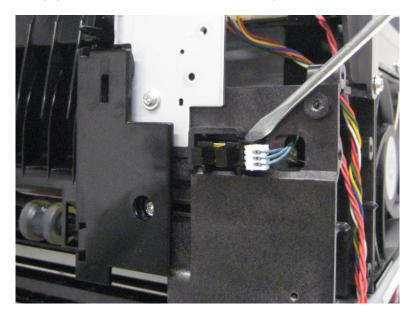
**Note:** It might take a small amount of force to remove the sensor (rear door interlock).
