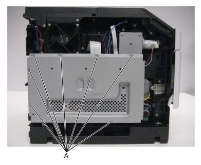
**3** Move the controller board access shield toward the front of the machine to remove it.
