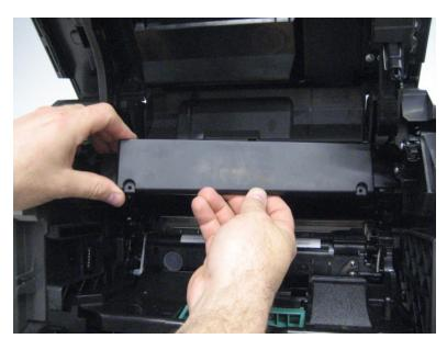
**5** Remove all of the harnesses from the back side of the printhead access cover.
