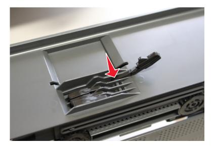
**b** Swing the actuator, and then press the free end to lock it in place.
