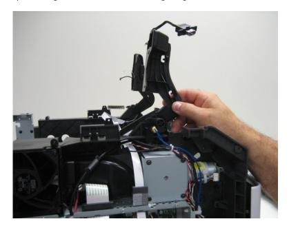
17 Remove the left control panel hinge.
