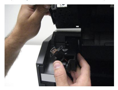
Disconnect any remaining grounding cables in the area of the left control panel hinge.
