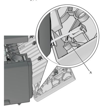
**Note:** Fasten the string to the rear side to prevent it from recoiling into the interior of the expander.
