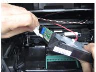
**Installation note:** When the new laser printhead has been installed, complete the polygon printhead mechanical registration adjustment procedure, as needed. See **"Polygon printhead mechanical registration adjustment" on page 274**.
