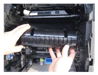
**Installation warning:** Ensure that the four retention hooks (A) on the inner guide deflector are properly reattached.
