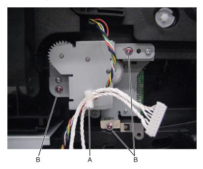
**Note:** When removing the lowermost screw, the grounding plate will become detached.
