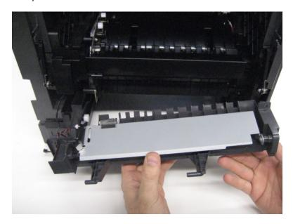
**Installation warning:** When replacing the MPF feeder lift plate, ensure that the MPF feeder lift plate cable and solenoid cable are properly rerouted and that all cables are properly reconnected. Make sure that these cables are not pinched between the MPF feeder lift plate and the frame before replacing the screws.
