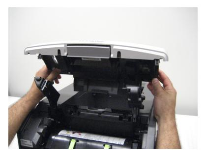
Remove the control panel front cover. See "Control panel front cover removal" on page 396.
