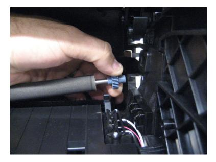
**Note:** When removing the transfer roller, avoid all contact with the foam surface, or print quality issues might occur.
