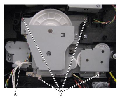
Remove the main drive motor from the machine.
