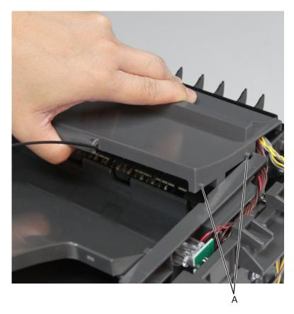
**5** Disconnect the solenoid cable (J2A, J2B, or J2C) from the controller PCBA.
