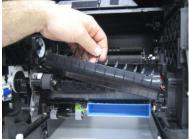
**13** Lift the right hinge point, and remove the duplex exit diverter.
