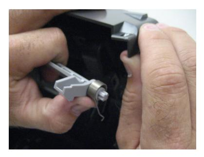
Carefully remove the control panel latch.
