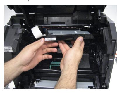
Disconnect the two cables from the laser printhead.
