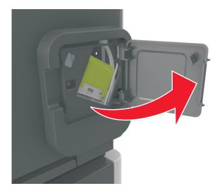
Pull down the latch of the staple cartridge holder, and then pull the holder out of the printer.
