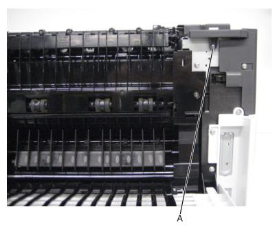
**3** Remove the output bin sensor cover.
