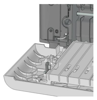
Remove the two screws (B), then remove the left cover.
