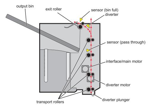
When the HCOE is installed on top of the printer, the diverter plunger changes the position of the diverter below it. Since the diverter position of the printer below is opened, the printed paper will be re-routed. Instead of exiting the standard output bin, the media enters the HCOE. The movement of the diverter plunger can be controlled by its diverter motor, depending on the printer's commands.
