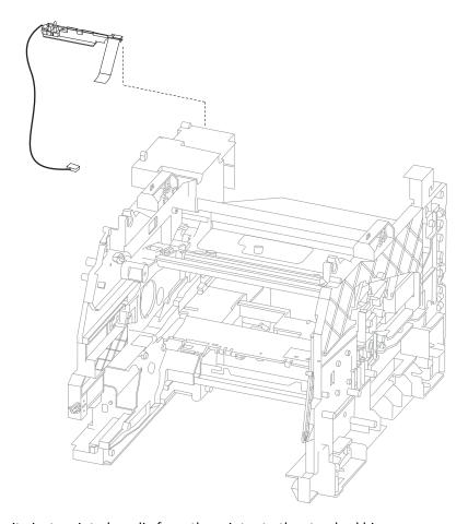
The standard media exit ejects printed media from the printer to the standard bin .
