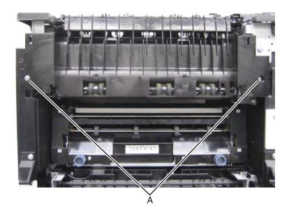
**5** Move the upper redrive down and away from the machine to remove it.
