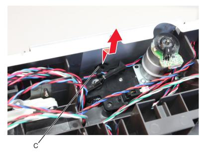
**Warning—Potential Damage:** Ease the media feeder off the drawer. Be careful not to damage the media feeder.
