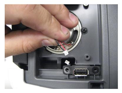
7 Disconnect the left control panel hinge, and remove the USB cable from the control panel.
