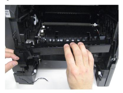
**Installation note:** When replacing the media turn guide, ensure that the alignment pin properly engages the media turn guide and that the alignment hooks properly engage the slots in the frame. If these parts are not properly engaged, paper jams will occur.
