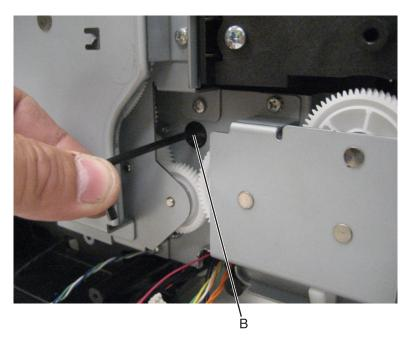
**Installation warning:** Make sure to reattach the grounding strap to the correct screw, and make sure the grounding strap is out of the paper path.
