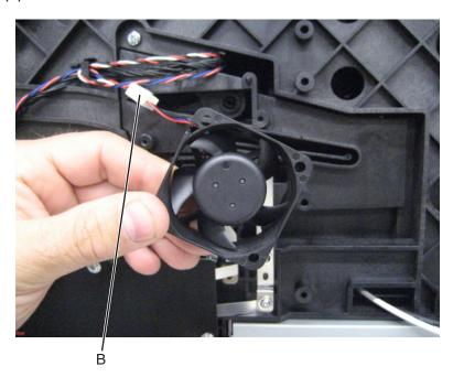
**Installation note:** When replacing the cartridge cooling fan, ensure that it is installed as shown in the picture.
