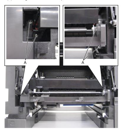
**8** Press down the plate, as shown in the following image, and remove the MPF feeder lift plate.
