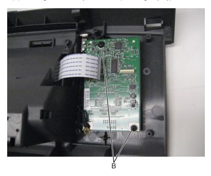
Remove the control panel board.
