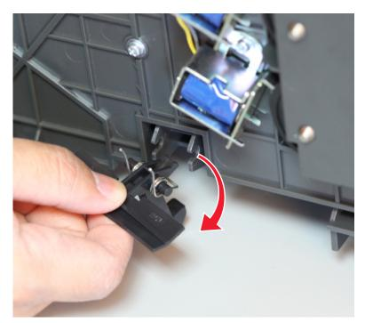
**5** Carefully lift the inner right frame, then remove the ground screw (B).
