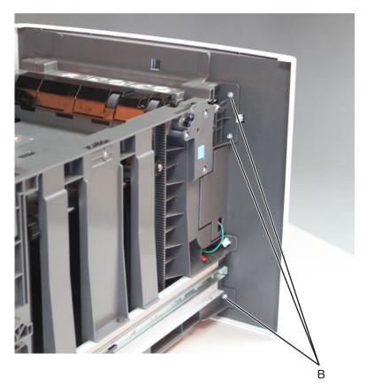
**4** Release the latches, and remove the media tray front cover.
