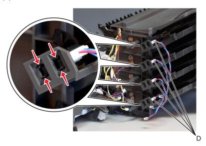
**9** Release the latches, and remove the sensor (bin full receive).
