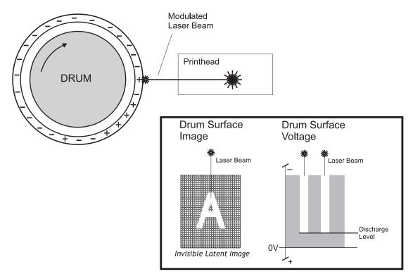
The Printhead generates a beam of laser light. Image data received from the controller board assembly modulates this beam, turning it on and off according to image information that is received from the host computer and software.
