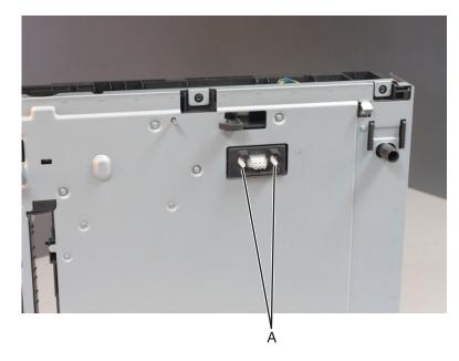
**6** Route the upper interface cable off the drawer, and remove.
