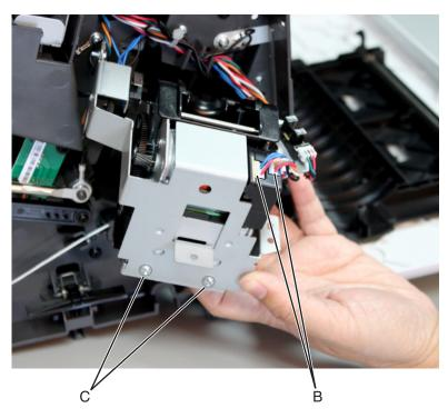
**5** Remove the stapler carriage assembly.
