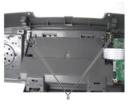
**9** Remove the 7" tilting display from the control panel.
