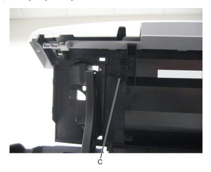
**8** Disconnect the left control panel hinge, and remove the USB cable from the control panel.
