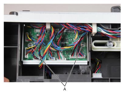
4 Remove the controller PCBA.
