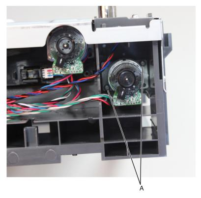
**5** Route the cable off the drawer, then remove the transport motor.
