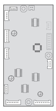
**3** Remove the three screws (A), then remove the controller PCBA.
