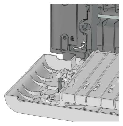
Position the door at an angle approximately 90 degrees from the expander, then remove.
