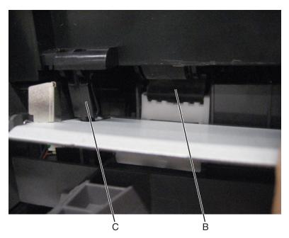
**Installation warning:** When replacing the MPF feeder lift plate ensure that the pick pad (B) is placed properly behind the MPF feed roller.
