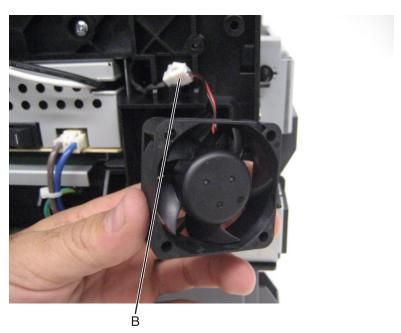
**Installation note:** When replacing the duplex cooling fan, ensure that it is installed as shown in the picture.
