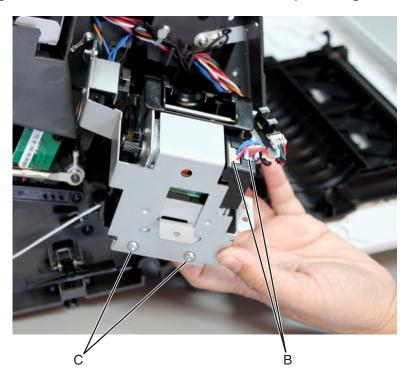
Lift the stapler carriage to access the screws securing the limit switch.
