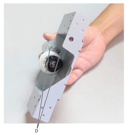
**6** Remove the tray lift drive motor.
