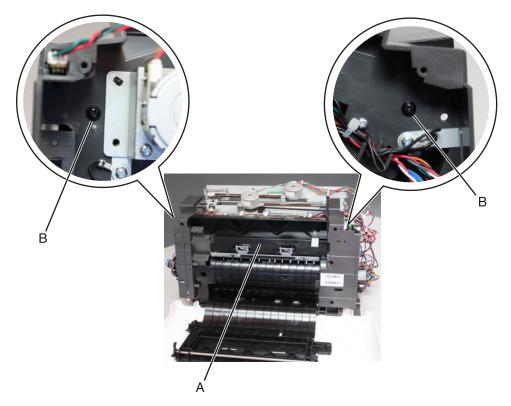
**5** Move the media stack flap to the right to release the pins from the holes.
