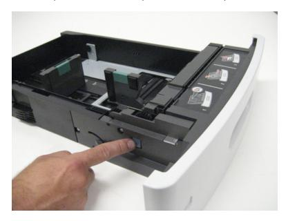
**3** Remove the separator roller assembly.
