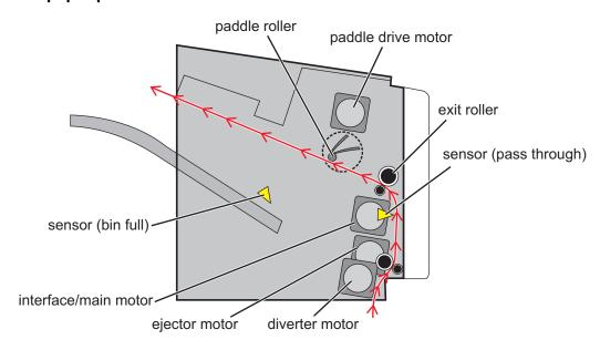
When the finisher is installed on top of the printer, the diverter plunger changes the position of the diverter below it. Since the diverter position of the printer below is opened, the printed paper will be re-routed. Instead of exiting the standard output bin, the media enters the staple finisher. The movement of the diverter plunger can be controlled by its diverter motor, depending on the printer's commands.
