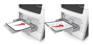
**Note:** When loading A6-size paper, make sure the multipurpose feeder extender rests lightly against the edge of the paper so that the last few sheets of paper remain in place.
