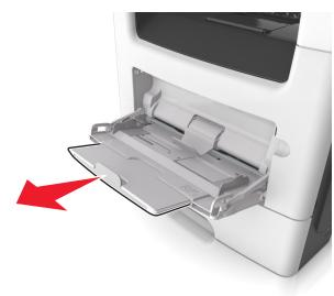
**b** Pull the extender gently so that the multipurpose feeder is fully extended and open.
