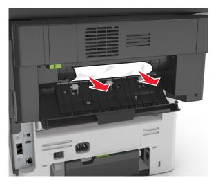
**3** Open the finisher narrow door, and then remove any paper fragments inside the narrow door.
