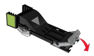
**5** Insert staple cartridge back into the finisher until it *clicks* into place.
