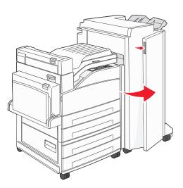
**2** Hold the lever on the staple cartridge holder, and move the holder to the right.
