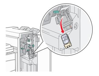
4 Use the metal tab to lift the staple guard, and then pull out the sheet of staples.Discard the entire sheet.
