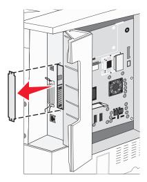
4 Align the connector on the internal print server or port interface card with the connector on the system board.Note: The cable connectors on the side of the optional card must fit through the opening in the faceplate.
