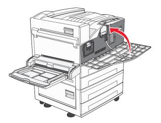
**Note:** After you insert the photoconductor and close all the doors, the printer performs a motor cycle and clears the Replace Photoconductor warnings.
