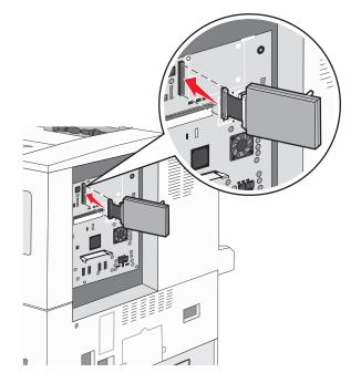
**6** Flip the hard disk over, and then press the three posts on the mounting plate into the holes on the system board. The hard disk *snaps* into place.
