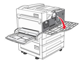
Note: The photoconductor cannot be pulled out if Side Door A is closed.
