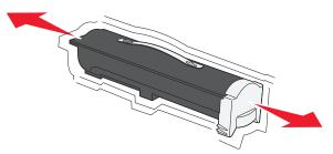
**6** Insert the new cartridge into the printer. Push the toner cartridge in as far as it will go. The cartridge *clicks* into place when correctly installed.
