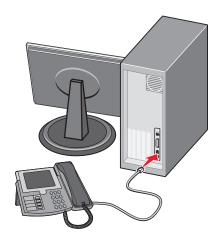
**6** Connect an additional telephone cord from the computer modem LINE port it to the printer EXT port i...
