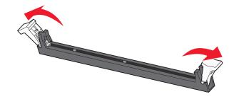
**4** Align the notches on the memory card with the ridges in the connector.
