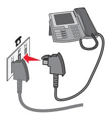
**5** If you would like to use the same line for recording messages on your answering machine, then connect a second telephone cable between the answering machine and the other N slot of the active analog telephone wall jack.
