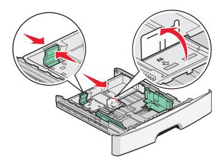
Note: Use the size indicators on the bottom of the tray to help position the guide.
