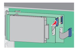
To install a printer hard disk directly onto the system board:
