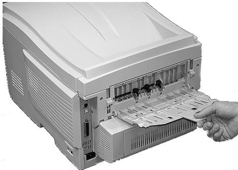
Open the face up stacker at the rear of the printer and pull out the tray extension.
