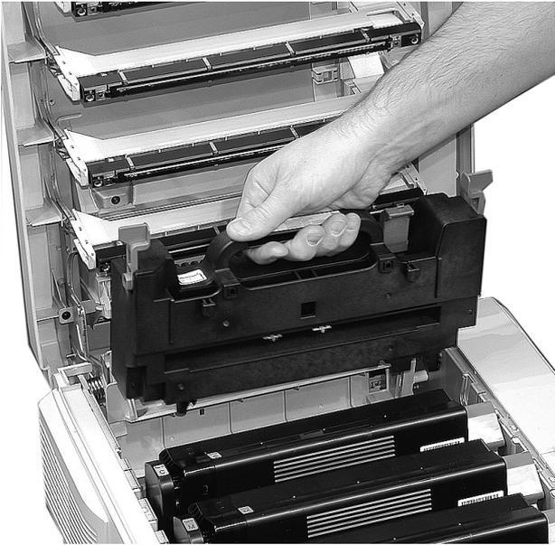
4. Remove the new fuser from its packaging. Remove any packing tape.
